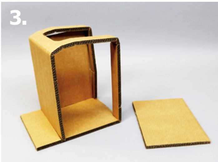
3. The template is then folded into its appropriate shape. The multiple parts of the standing frame are then assembled and reinforced using Elmer's glue, hot glue, and sharpened wooden dowels that are driven down into the cardboard.
