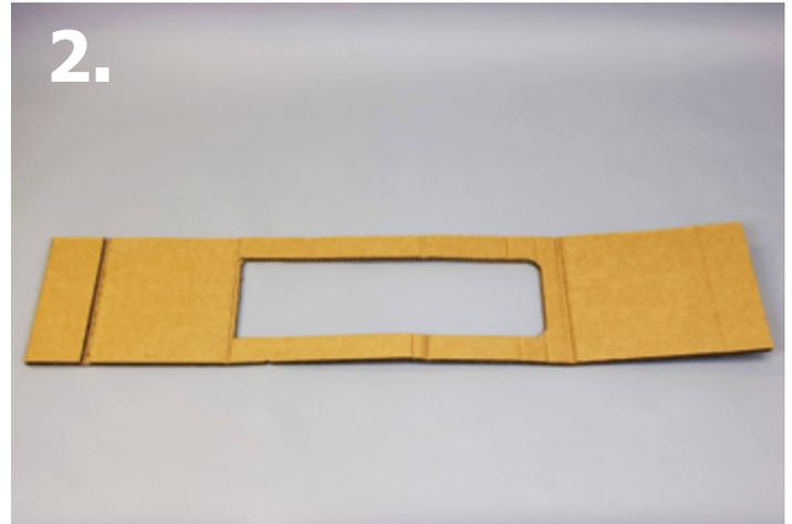
2. Bend marks are indented using the back edge of a spoon. The pattern is bent in the appropriate spots using a straight edge ruler or the side of a table. A groove is created by removing two layers of cardboard with a precision knife to create a male/female joint.
