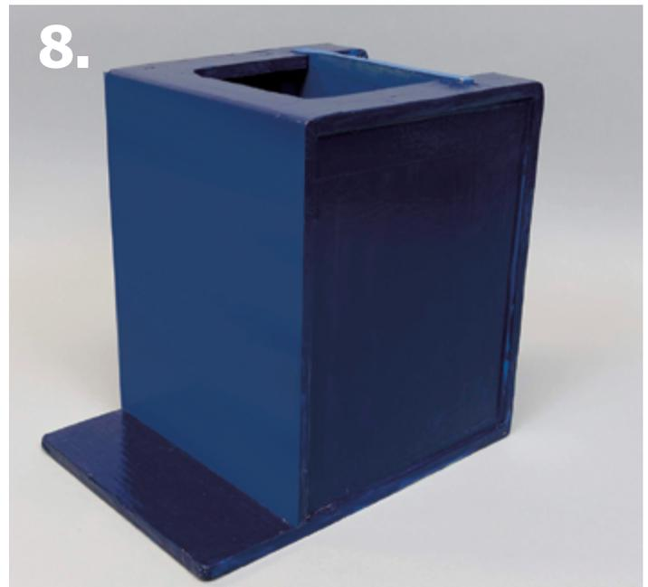
The entire device is then primed, painted, and polyurethaned to add to its aesthetics, rigidity, and resistance to water and wear and tear.
