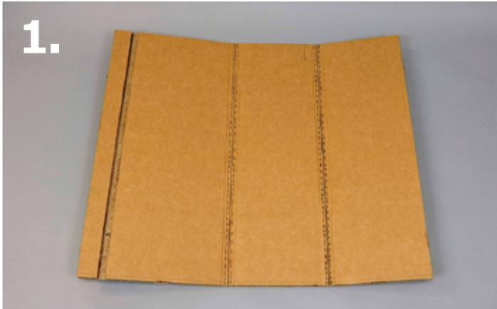
The pattern of the calendar board is drawn onto a sheet of tri-wall cardboard and cut out using either a utility knife, jig saw, or band saw. Lines are marked on the template to show where bends and scores will be made. Bend marks are indented using the back edge of a spoon. The pattern is bent in the appropriate spots using a straight edge ruler, or the side of a table. A groove is created by removing two layers of cardboard with a precision knife to create a male/female joint.
