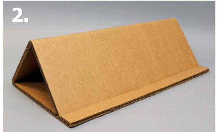
The template is then folded into its appropriate shape and glued into place. The front and rear faces of the calendar frame are at an angled, upright position. This will bring the visuals that will eventually be placed on top into the user's field of view where they can be seen more easily.
