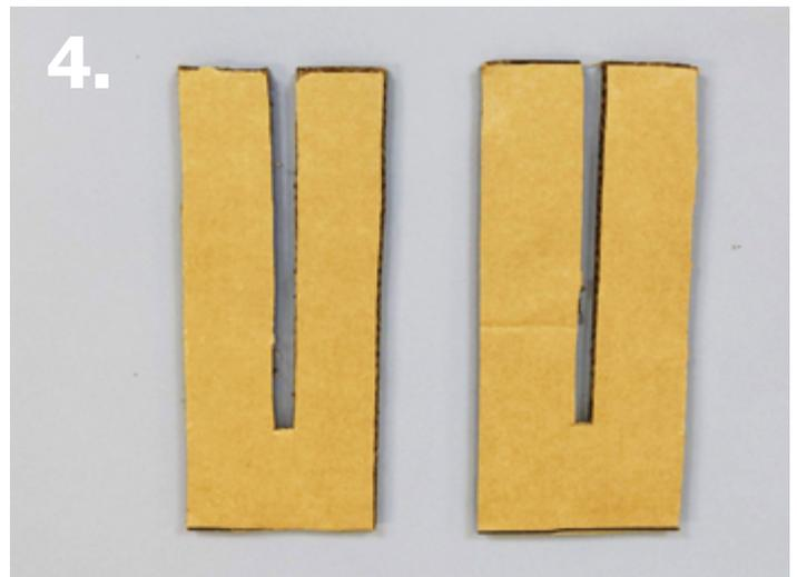
4. Separate pieces are cut out for the slot mechanism that will be used to hold the child upright within the standing frame.
