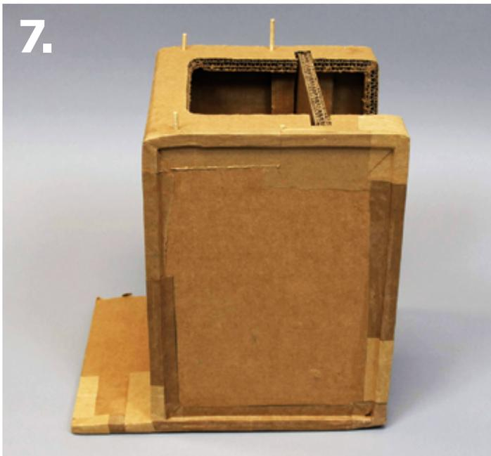
Heavyweight paper applied with Elmer's glue is used to cover the exposed corrugate edges of the device, holes where dowels were driven through, and any other torn or punctured areas of the cardboard.
